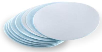
Polycarbonate track etched PC TEM has a smooth surface and controlled pore structure for capturing organisms and particulate on the surface. It's often the filter of choice for direct staining and microscopic examination, or concentrate and elute methods like *Legionella* testing. Also used in sample concentration and bead-beating for PCR sample prep.
